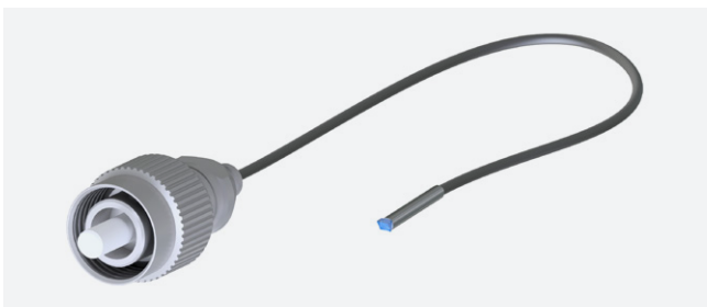
Fiber-optic assembly of 1.0 mm GRIN-lens with 90° prism, mounted in 1.2 mm stainless steel tube, fiber in 0.9 mm tubing with FC-connector
