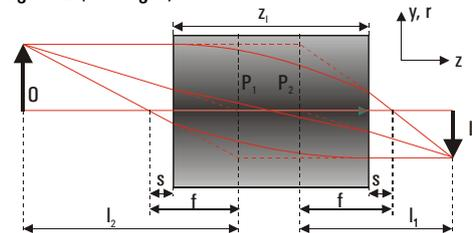
Fig. 4. Image formation by a GRIN focusing lens
