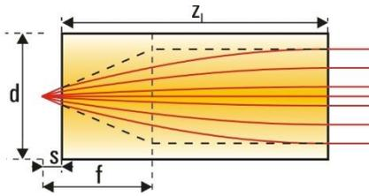
Gradient index lenses for fiber coupling and beam shaping of laser diodes
