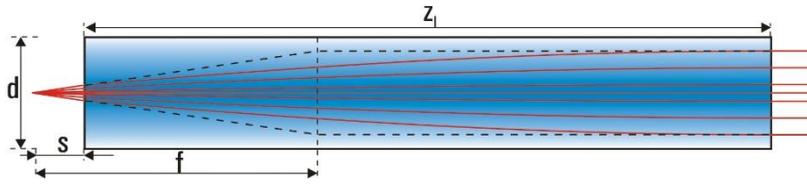
Gradient index lenses for fiber coupling and beam shaping of laser diodes
